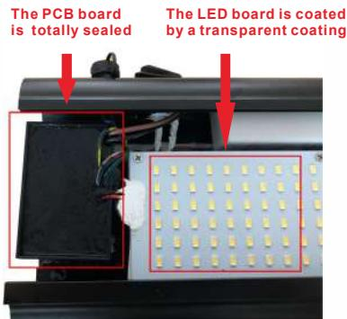
The enclosure of it is sealed, and the PCB board is totally sealed, so the electron components will not contact with corrosive air and moisture.
