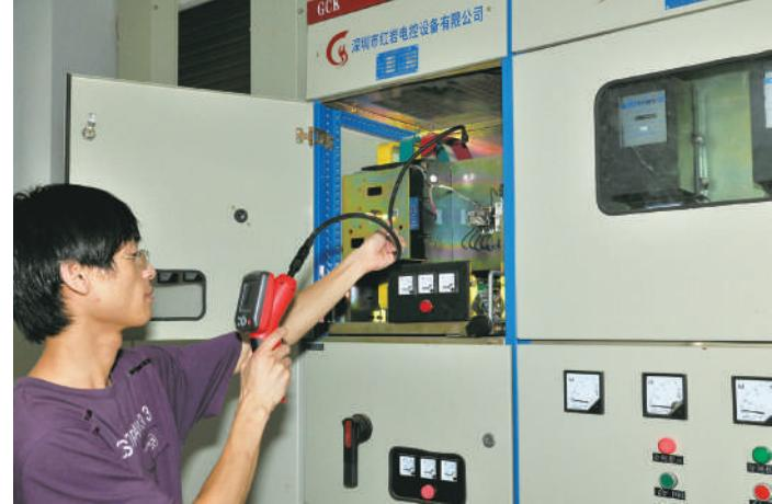
This high-definition video borescope has 2.4 "TFT LCD, Resolution: 480 (W) X234 (H), applying H.264 video codec technology makes images clear and exquisite, and equipped with curved waterproof goose-shaped tube which is a meter long, it will be easy to detect the object that cannot be touched and can't be visible by naked eye, meanwhile, access to AV video display and the signal system can be derived in both NTSC / PAL formats and can switch the signal format automatically.
