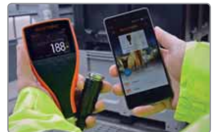
USB and Bluetooth® data output to iPhone or Android™ devices
