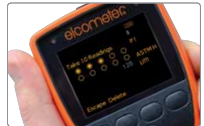
Select 5 or 10 readings per measurement
