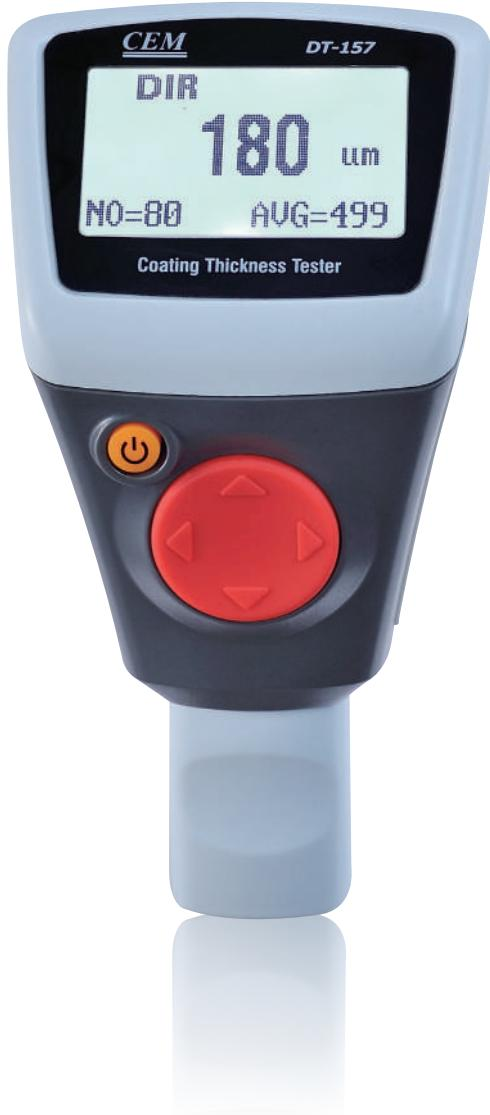
The coating thickness gauges work either on the magnetic induction principle or on the eddy current principle, depending on the type of probe used. You can select the type of probe via MENU system, or it will work automatically.
