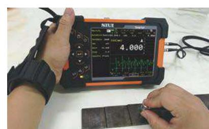
Thickness measurement on step block
